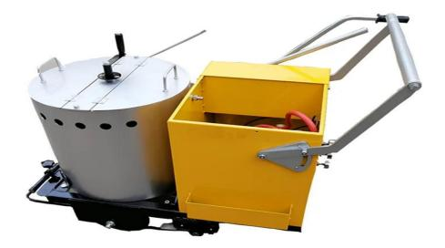
Thermoplastic Road Marker Applicator Machine (Line thickness: 1.0-2.5mm; with complete accessories (glass beads dispenser, indicative rod, etc.); Lane marking width: 100m, 150mm,200mm and 300mm; Hand-push; Paint tank capacity: 100kg; heating method: LPG, w/ 1year warranty)
